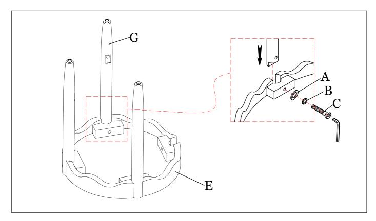
STEP 2: Attach bottom Shelf (F) and Leg (G) on the Table of Step 1 by using Flat washer (A), Lock washer (B), Bolt (D) with Allen key.
